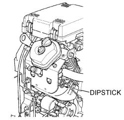
Figure 6. Engine Oil Dipstick Removal
